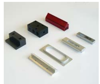
↑ Some examples of finished components from brass, aluminium and steel.
