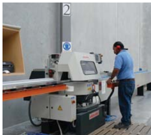
↑ Elumatec digital cutting saw. 10m roller beds for the longest extrusions.
