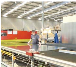
↑ 3m wide guillotine and table. 6x2m aluminium sheet stock in background.
