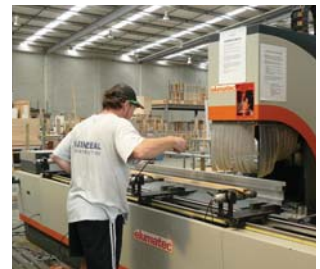
↑ Elumatec long bed milling machine for accuracy on long lengths up to 7m.
